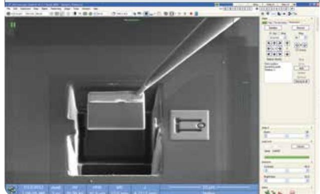
↑ Control of the EasyLift is integrated into the DualBeam UI. Movement of the probe can be done on screen with the mouse.
