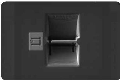
← Sample transferred to the TEM Grid with fine precision movement
