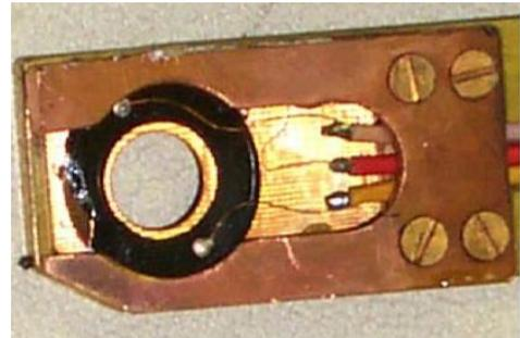
Figure 2. Yttrium aluminum garnet (YAG) backscatter detector.
